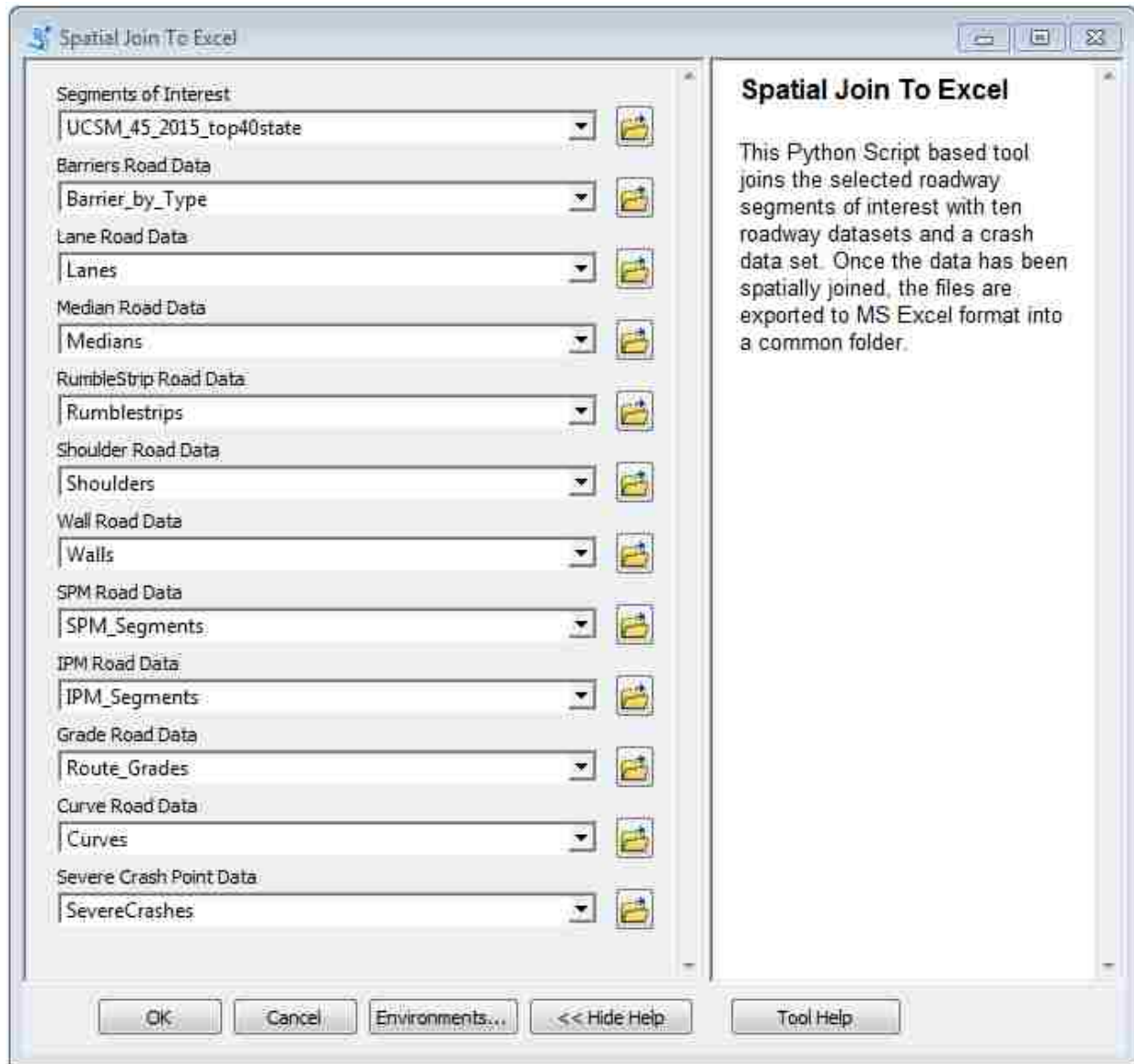
Figure 7-24: “Spatial Join to Excel” ArcMap tool to spatially join roadway characteristics and crash data with selected roadway segments.
